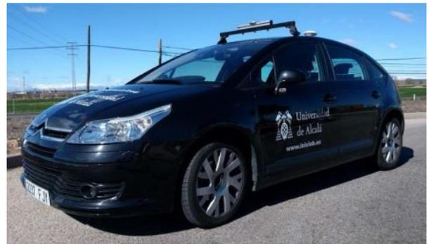
DRIVERTIVE on-board sensors (vision, laser and radar).
